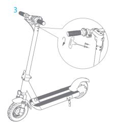
3.Use the hexagon wrench in the box to tighten the screws on both sides and the back of the IOT lower cover
