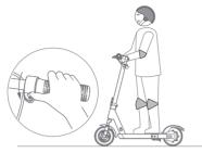
3 Put your other foot on the footrest to keep both feet stable. Press the throttle on right hand to speed up when you are balanced.Note, for your safety, the motor will not engage until the scooter reachs 5km/h
