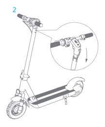
2.Install the handlebar into the stem tube.
