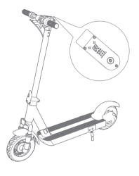
1 Power on the scooter and check the indicator lamp power level. Charge the scooter if the battery level is low.
