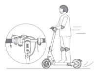
4 Slow down by releasing the throttle, hold the brake lever in order to make a brake, please note that the rear fender is not a mechanical braking and do not stamp it with foot while riding.
